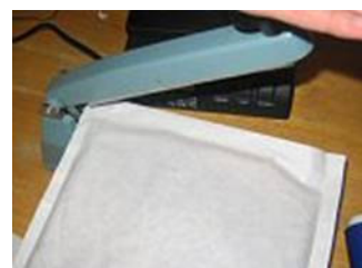
Sealing the 'envelope' with the impulse sealer.
